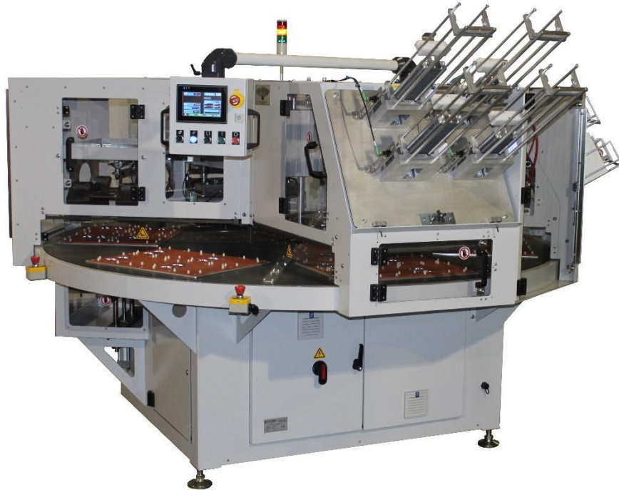
FAB/PH Rotary Blister Sealing Machine shown with 4-cavity sealing fixtures
